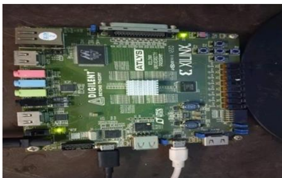
Figure 7: FPGA Spartan 6 hardware snapshot
