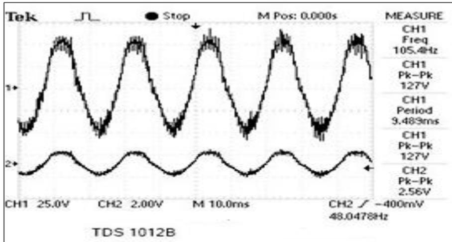
Figure 17: SAPF Compensated Voltage and Voltage at Current at Source Side
