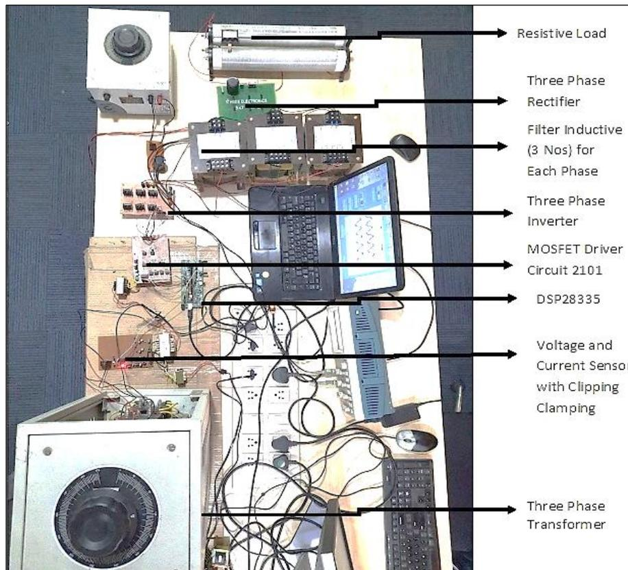
Figure 5: Experimental Setup-Schematic of the System
