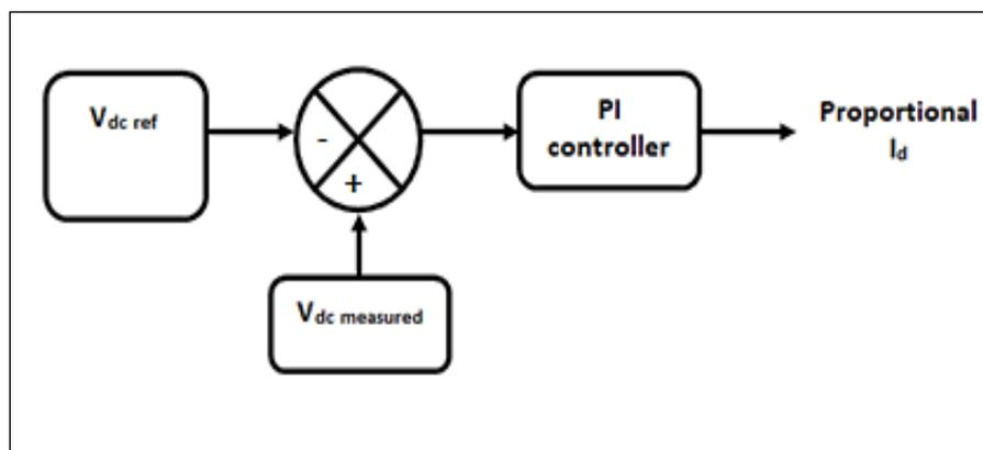
**Figure 2:** Block Diagram of PI Controlled DC Link Voltage Regulator
