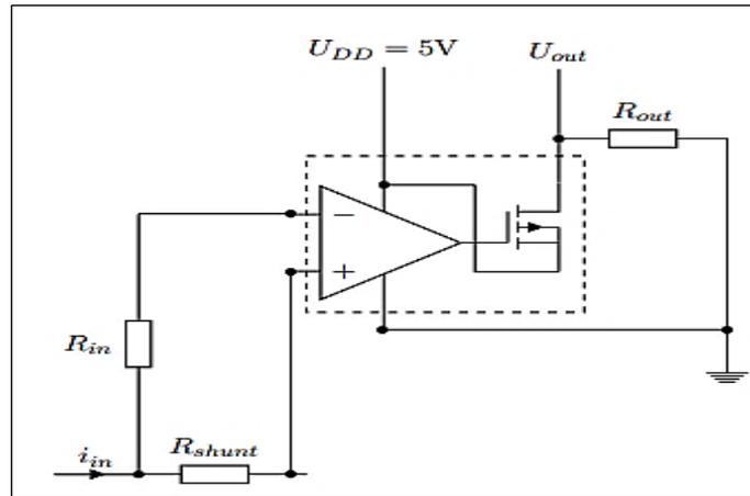
Figure 6: Circuit Diagram of Current Sensor
