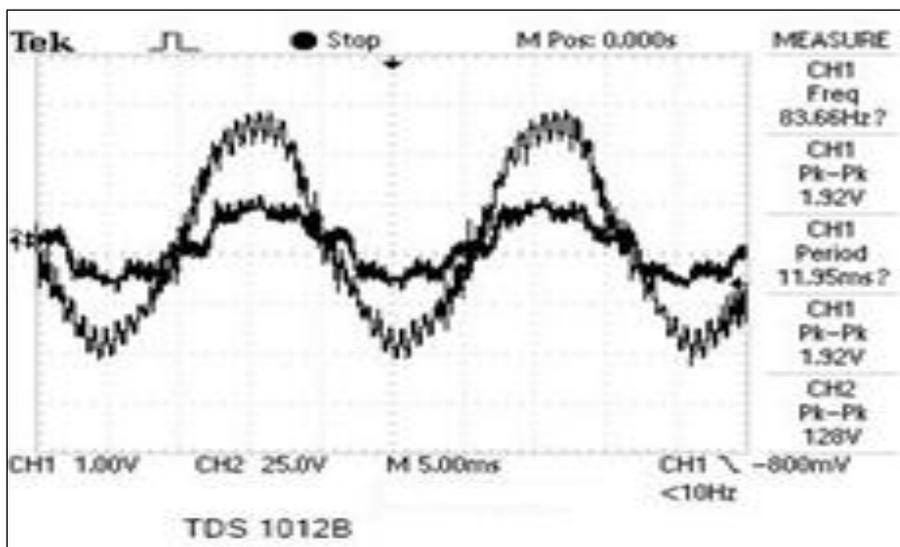
Figure 16: Voltage and Current with Nonlinear Load (Rectifier Load)
