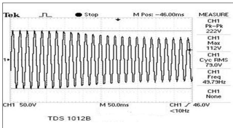
**Figure 13:** Real Time Fault Detection Out from DSP ePWM Pins for Sag Fault
