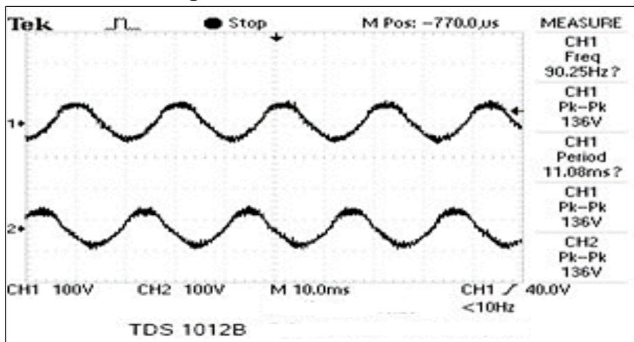
Figure 19: Phase B and C Voltage at Source Side
