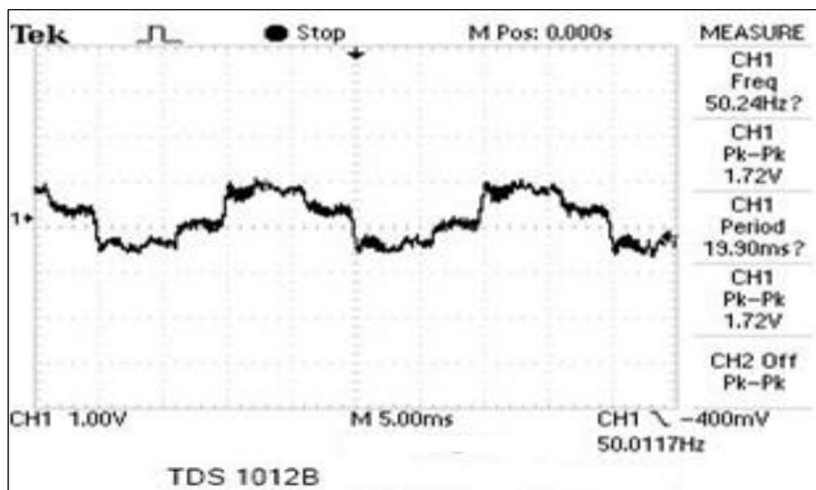
Figure 15: Rectifier Load Harmonics Response in Current (Phase A)
