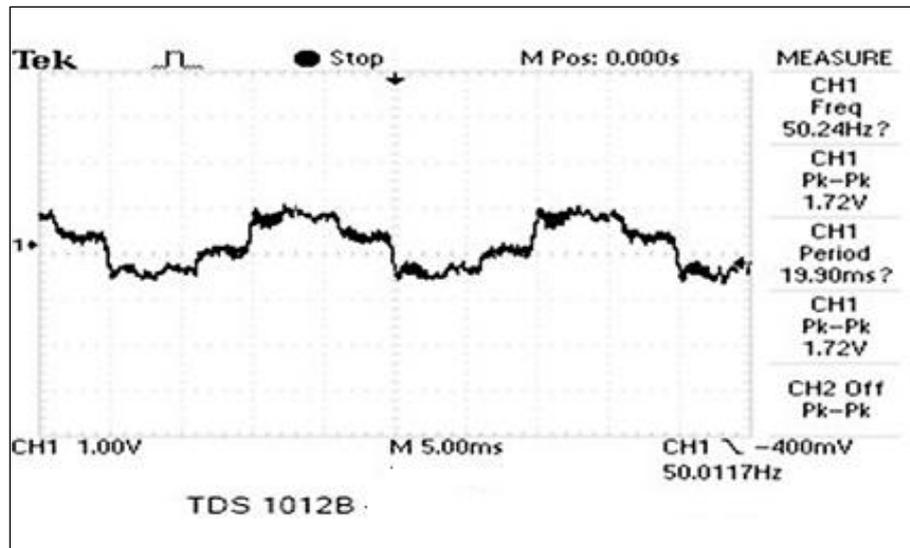
**Figure 12:** Real Time Fault Detection Output from DSP ePWM Pins for Harmonics Fault
