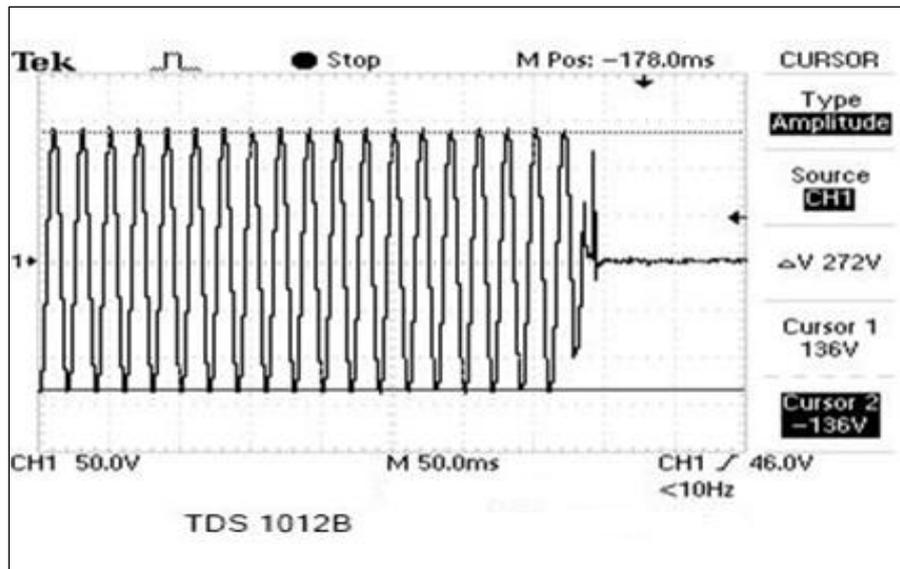
Figure 14: Real Time Fault Detection from DSP ePWM Pins for Interruption Fault
