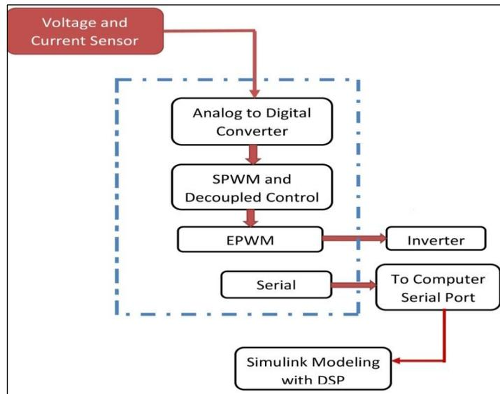
**Figure 10:** Overall Block diagram – SAPF Emulation Using Hardware in Loop (HIL) Implementation Using MATLAB
