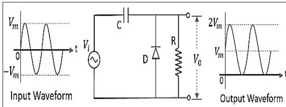
**Figure 9:** Circuit Diagram of Clamper
