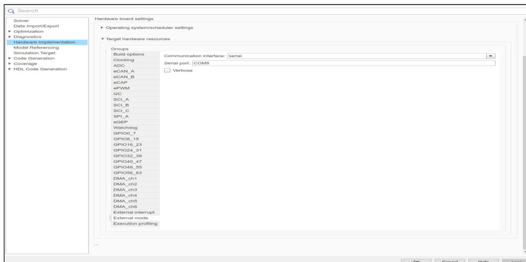
**Figure 11:** Hardware Implementation External Mode in COM8
