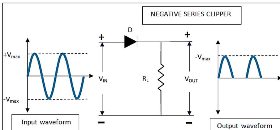
Figure 8: Circuit Diagram of Clipper
