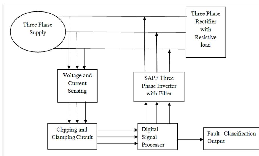
**Figure 1:** Schematic Diagram of Proposed System
