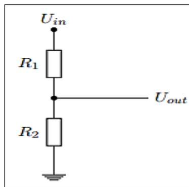
Figure 7: Schematic Diagram of Voltage Sensor
