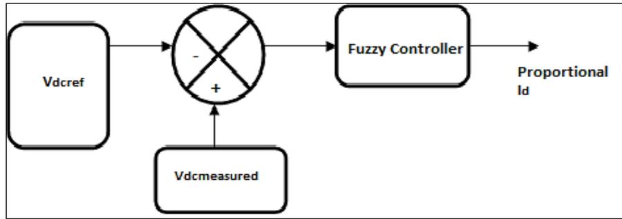
**Figure 3:** Schematic Diagram of Fuzzy Controlled DC Link Voltage Regulator
