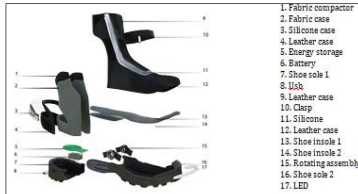
Figure 3: Exploded View of Military Boot
