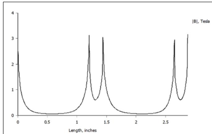
**Figure 10:** Magnetic Flux Intensity along the Circumference of the Bot
