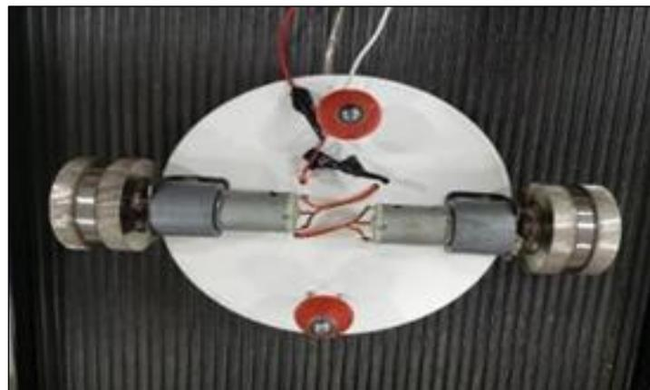
**Figure 13:** Actual Fabrication of Omni Bot
