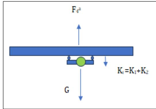
Figure 4: Case 4: Bot-Upside down Inverted Surface
