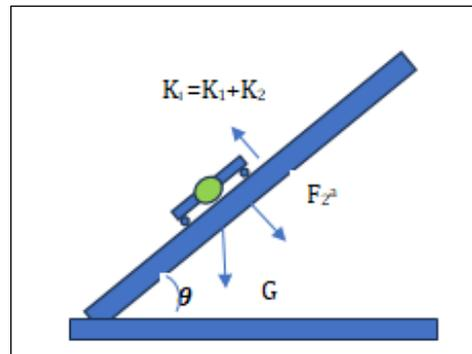
Figure 2: Case 2: The Bot on Inclined Surface
