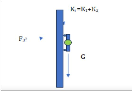
Figure 3: Case 3: The Bot on Vertical Wall
