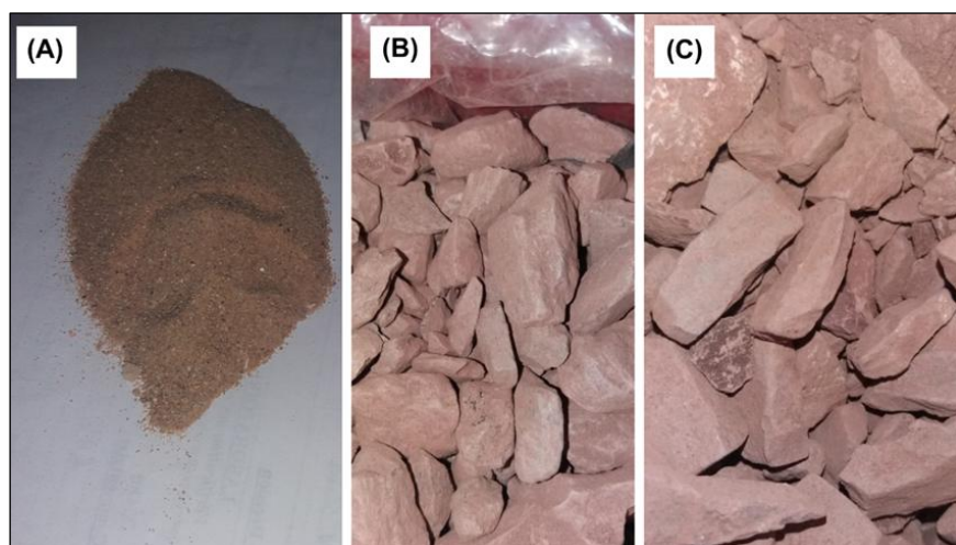
Figure 1 : Raw Materials for Ceramic Production : (A) LOPT (Lead Ore Processing Tailings), (B) Clay 1 (CL1), (C) Clay 2 (CL2)
