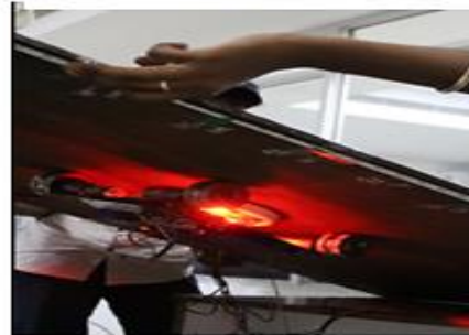
Figure 15: Bot at Obtuse Angle (120°) With Active SAM Carrying Overcoming Rollover
