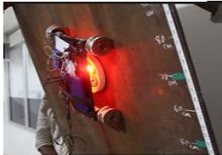
Figure 14: Bot at Obtuse Angle (105°) With Active SAM Carrying Overcoming Rollover
