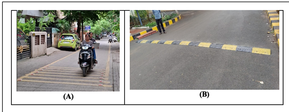
Figure 5: Road Profile Used for Vibration Testing: (A) Rumble Strip Road Profile, (B) Speed Bump Road Profile
