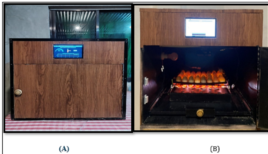
Figure 6: Actual Design of the Fabricated IoT-based Smart Egg Incubator: (A) Exterior View, (B) Interior View
