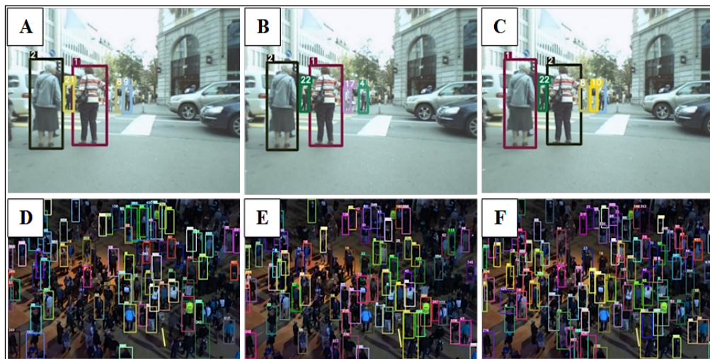
Figure 3: ByteTrack Tracking Examples on MOT17 and MOT20 Under Different Scene Conditions. (A) MOT17-05 with YOLOv3-tiny, (B) MOT17-05 with YOLOv5n, (C) MOT17-05 with YOLOv8n, (D) MOT20-05 with YOLOv3-tiny, (E) MOT20-05 with YOLOv5n, (F) MOT20-05 with YOLOv8n
