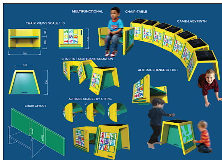
Figure 6: Views of Chair-Table Modules, Constructive Connection Nodes, Three-Dimensional Images of Application Options
