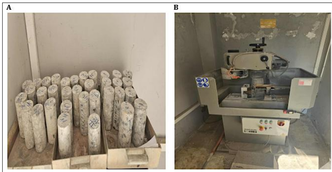
Figure 2: Specimen Preparation Process. (A) Extracted Class B30 Concrete Core Specimens (7 Cm X 14 Cm), (B) Precision End-face Grinding Machine
