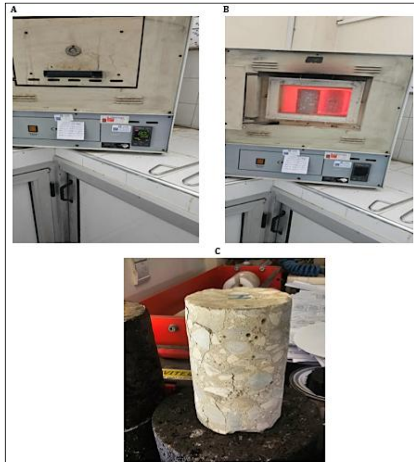
Figure 3: Thermal Exposure and Physical Degradation of Concrete Test Specimens. (A) Concrete Specimen During Thermal Exposure At 800 °C Inside the Muffle Furnace, (B) Concrete Specimen Undergoing Cooling at Ambient Room Temperature, (C) Microstructural Cracking and Surface Deterioration After Extreme Thermal Exposure
